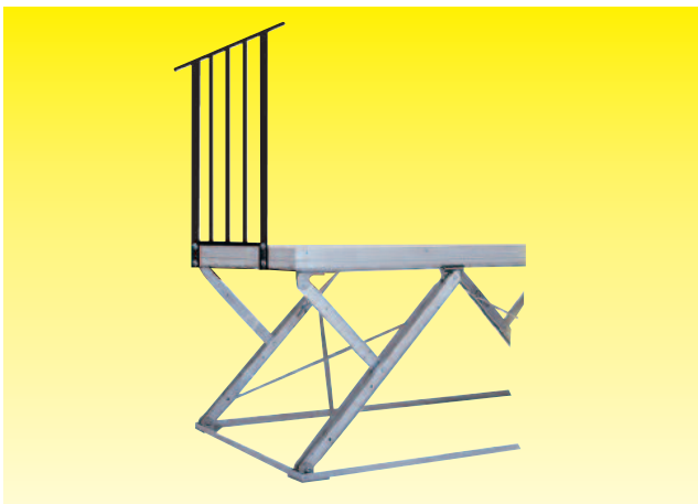
Safety railings in accordance with DIN 4112 standard for scissor-type platforms made of tubular steel, black powder coated, other colours on request.
