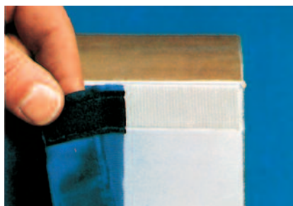
Setting of the textile masking with Velcro tapes.
