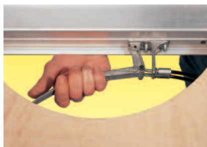
Height adjustment by means of Bowden cable system.
